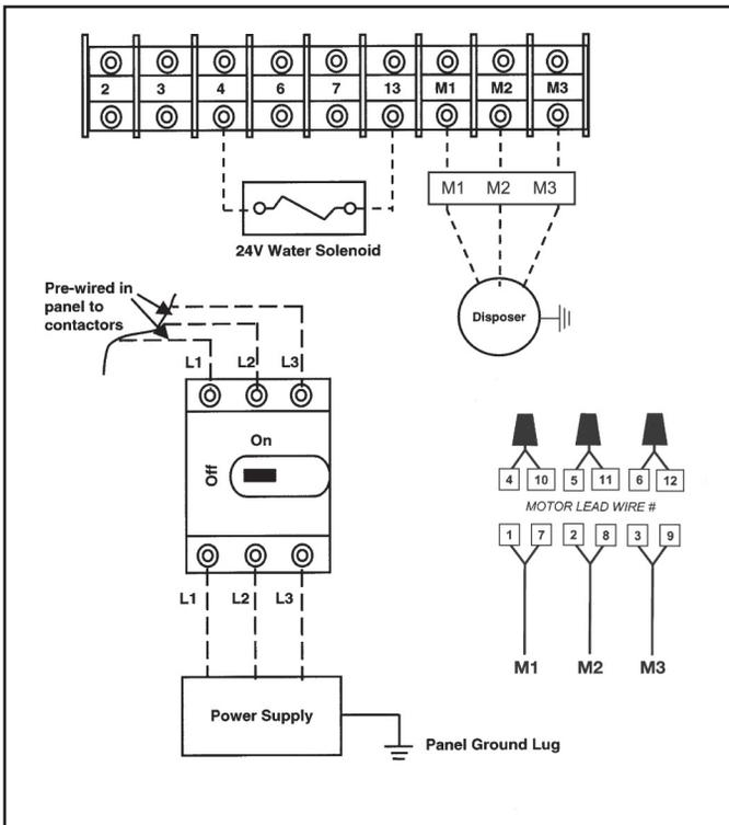
Figure 5. Incoming 208-240 V Three Phase Line Power
