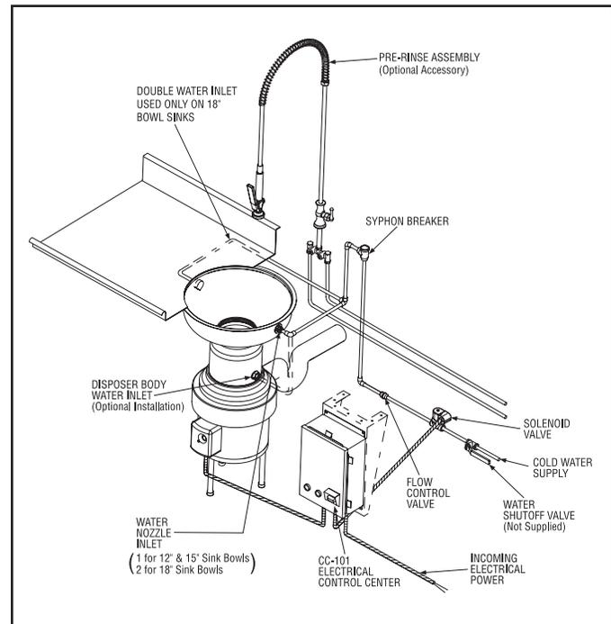
Figure 2. Typical Installation Diagram
