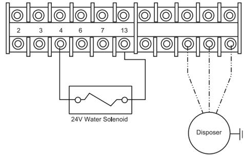
Figure 7. Water Solenoid Valve Wiring
