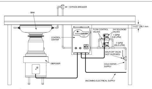
NOTE: The AquaSaver® control center should be mounted 1-1/2" (38.1 mm) back from the front surface of the table.
